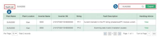
Step 3 Click Plant Name on the right side of Fault List. Select a target string and view Contrast analysis on strings for IV curve.
